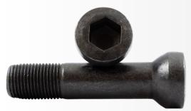
All **LoPro**® Bolts will have a tapered head. Overall length is used when measuring bolt size. A 1/2" Allen is used to tighten and remove. The **LoPro**® bolt will have an extraction slot at the end of the bolt for easy removal in case of breakage.
