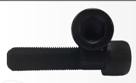
All Cap Screw bolts will have an internal hex head. Bolt length is determined by measuring the shank length below the bolt head. A 1/2" Allen is used to tighten and remove. The Cap Screw bolt will not have an extraction slot at the end of the bolt to aid in removal in case of breakage.
