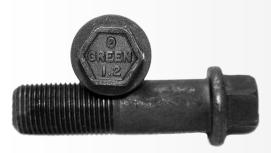
All **Greenbolt**® bolts will have a hex head. Bolt length is determined by measuring the shank length below the bolt head. A 5/8" Socket is used to tighten and remove. The **Greenbolt**® will have an extraction slot at the end of the bolt to aid in removal in case of breakage.
